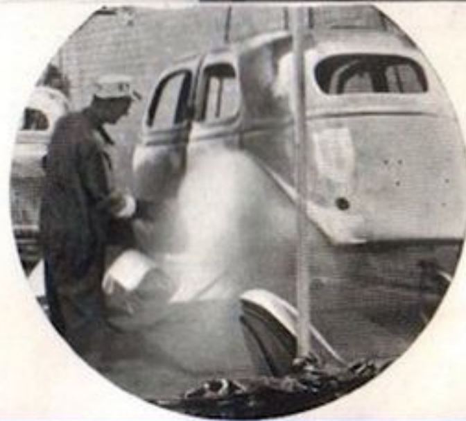
(Above) Sections of the paint division showing bodies and cabs on the overhead mono-rail conveyor undergoing various painting operations.
