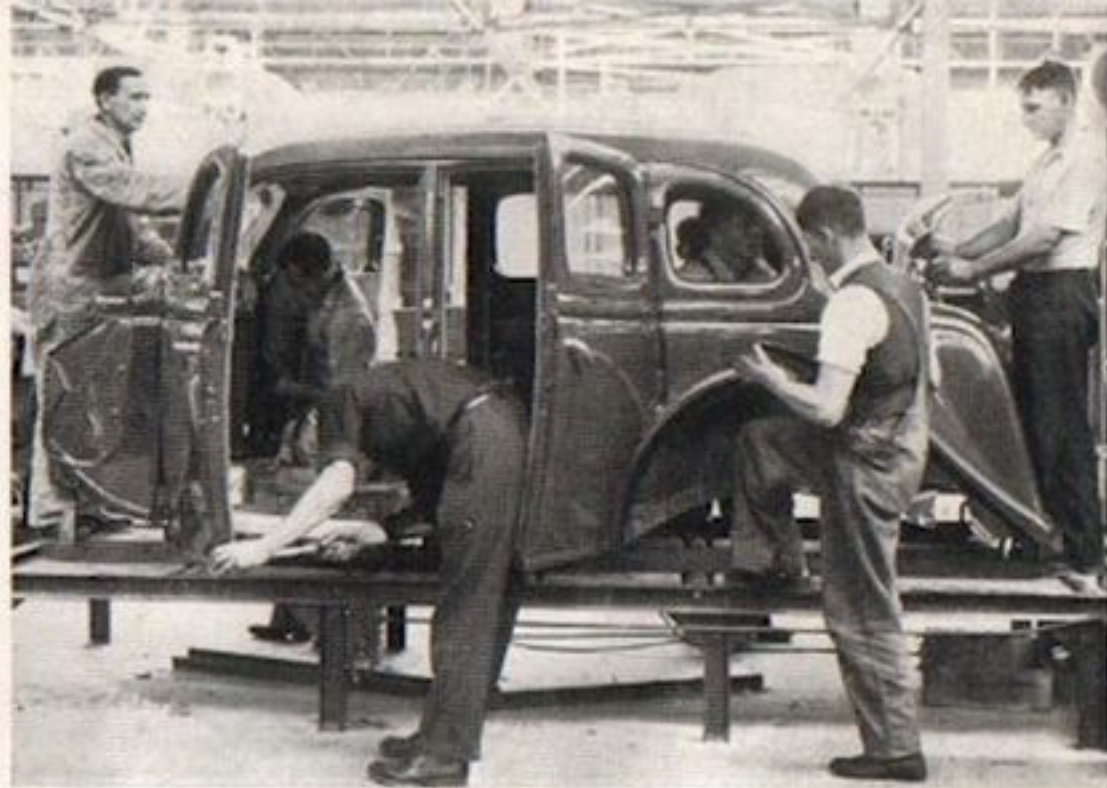
(Above) Door and window fittings, the safety glass, locks, dash and other appointments are added at the end of the trim line conveyor. The body is now ready to be fitted to the Chassis.
