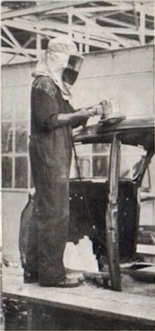
Every protection is provided for the workers throughout the factory as witness the operator of an electric sander shown above.
