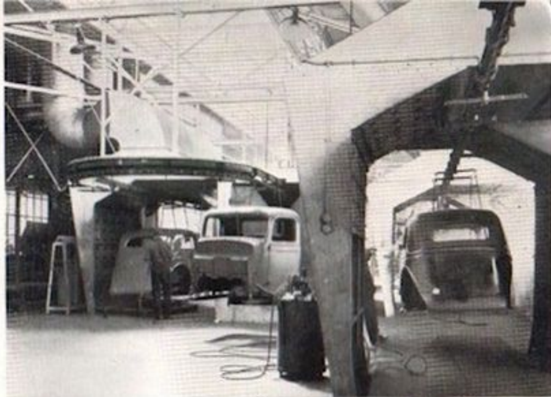
(Above) Sections of the paint division showing bodies and cabs on the overhead mono-rail conveyor undergoing various painting operations.
