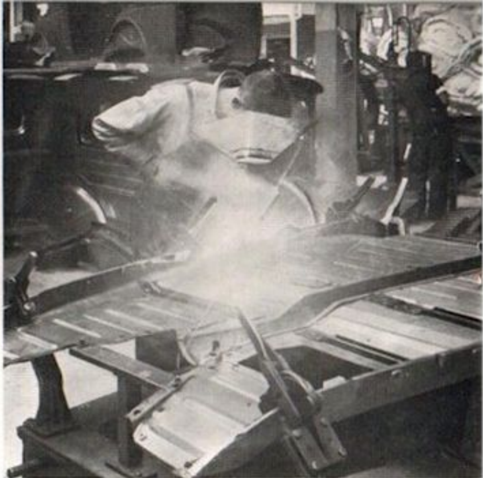
Special jigs hold the all-steel floor in position while it is welded into one piece amid a shower of sparks.
