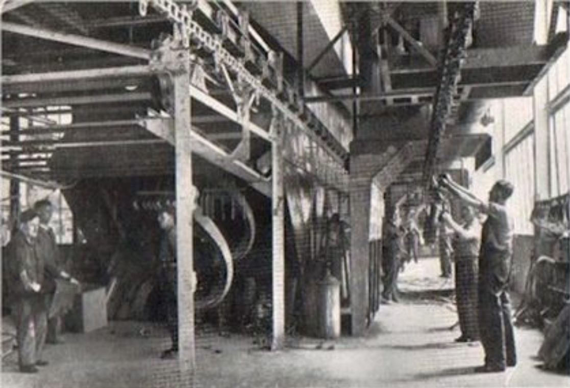
(Above) The Fender oven and overhead conveyor where wheels, hubs, fenders and all other small parts are enamelled and baked.
