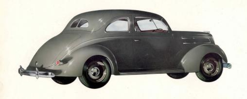
**THE CLUB COUPE** A splendid car for business or professional use. The new-type body accommodates six passengers inside and with the rear seat removed is easily converted into a single seater commercial type Coupe with maximum luggage carrying space. All Steel Body—one-piece steel roof, steel sides, and floor. V-type windscreen and all windows of Safety Glass. A rising type front seat with a dual range of adjustments. An ideal Business Coupe—smart, comfortable, efficient.
