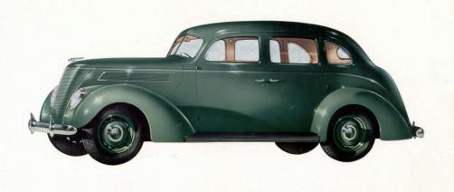
**THE TOURING SEDAN** A big, roomy, comfortable sedan of modern, stylish design. All-steel body with one-piece steel roof, steel sides and floor. Safety Glass in the new V-type windscreen and all windows. New design large-capacity luggage trunk. Interiors designed for maximum riding ease with deep restful upholstery. Front seat is adjustable. This V-8 model will appeal to business executives, salesmen and other commercial users as well as private owners.
