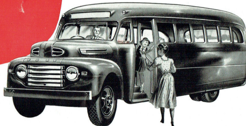
BUS CHASSIS, 14,500 lbs. G.V.W.—173" & 194" w.b.—Up To 27-Passenger
