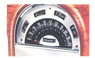
Smartly-Designed Instrument Cluster combines all instruments in one easy-to-read group, wherein lighting can be dimmed if desired.
