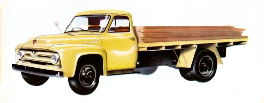
**ENGINE:** No. of cylinders—8. Bore and stroke—3.625 x 3.10 ins. Displacement 256 cu. inches. Compression ratio—6.7:1.
