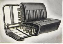
SEAT CONSTRUCTION. Ford's special seat construction includes special non-sag springs on rigid frames ensuring longer life and comfort. Deep upholstery is covered in longwearing Vinyl that can be washed easily.
