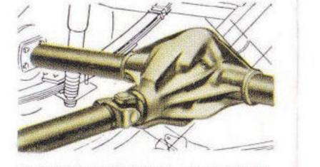
Ford's Hotchkiss drive eliminates excess weight and allows driving and braking forces to be transmitted through rear springs for smooth starts and stops and level-riding comfort.
