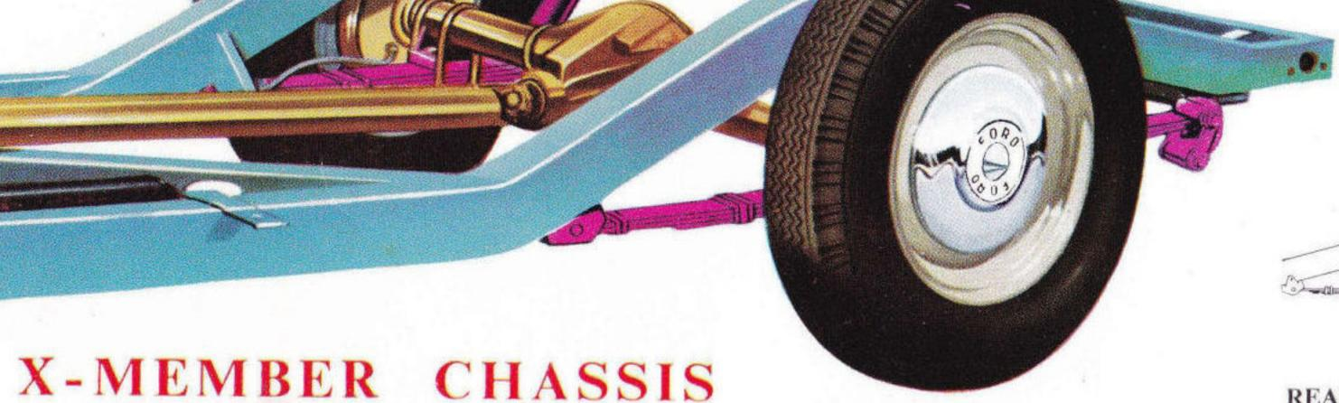
In this husky chassis you find still further reasons why Mainline is so **practical** a Coupe Utility. Deep, box-section frame members . . . massive X-member for big safety margin in resistance to torsional stress . . . everywhere you see strength. And, from balanced-ease steering to diagonally mounted shock absorbers, feature after feature contributes to smoother, road-hugging stability. Mainline's chassis is a solid basis for hard work.
