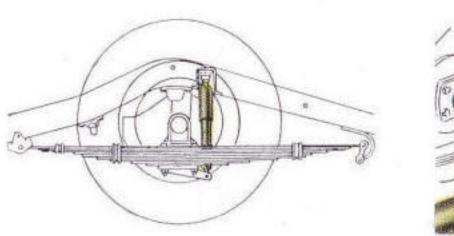
REAR SUSPENSION. Tension-type shackles at rear of springs result in a "variable rate" spring effect—soft, easy action over little irregularities, and a stiffer action for more control over big road pumps.
