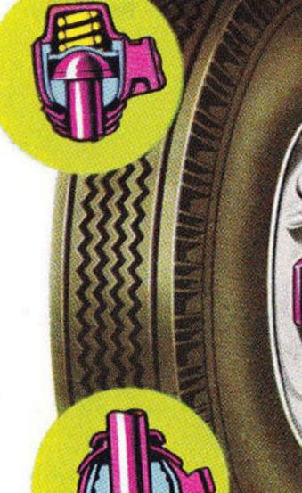
feature puts new pleasure and ease into driving . . . makes travel safer . . . cornering steadier . . . and rough going smoother. Movement of wheels is controlled through ball-joints, whether in up-and-down motion, or in steering motion when wheels turn left or right. Ball-joint Suspension is tilted, in effect "angle-poised," to absorb road shocks from the front as well as up-and-down.
