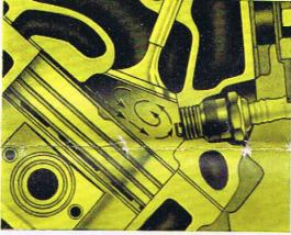
High-Turbulence Combustion. Wedge-shaped combustion chambers provide high-turbulence in the fuel-air mixture, giving more complete and efficient combustion without detonation, greater power output and thoroughness in scavenging of exhaust gases.
