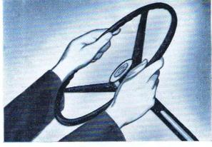
New Lifeguard steering wheel a Ford first. Deep-centre design allows safety of greater absorbing of impacts.
