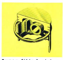
Super-fitted pistons. Flat head, autothermic design of light-weight aluminium alloy. 3 rings with chrome plating of top ring and phosphate-coated bottom ring has steel expander for closer oil control.
