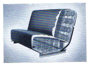
Wide-comfort seat . . . special construction absorbs road-bounces and longlife upholstery resists hard usage . . . seat keeps shape, and comfort lasts longer.
