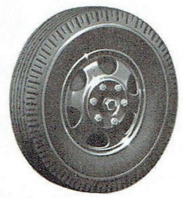
6-stud wheel In every way Ford builds stronger to last longer. For instance, on the heavy duty F600 models there is an increase in strength and safety even in wheel stud design, 6 studs are used to ensure strength and safety margins over and above stress and strain of loaded weight and road conditions.
