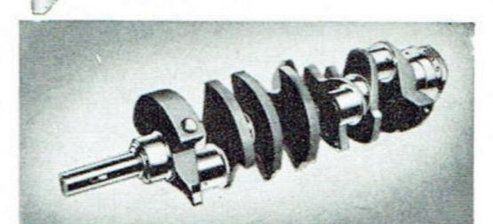
**Exceptionally Rigid Crankshaft** cast by an exclusive Ford method from a special iron-alloy, has 5 main bearings and eight integral counterweights for smoother operation and longer engine life.
