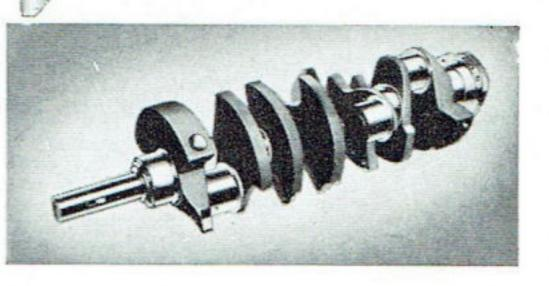
Exceptionally Rigid Crankshaft cast by an exclusive Ford method from a special iron-alloy, has 5 main bearings and eight integral counterweights for smoother operation and longer engine life.
