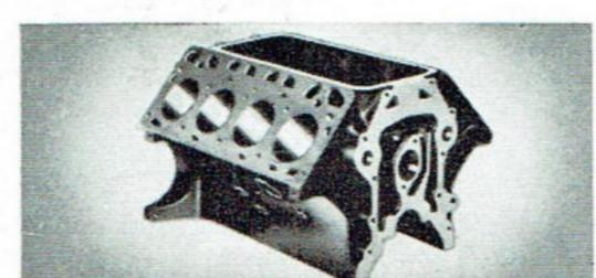
Deep Y-Block with its great rigidity means longer life, and smoother operation. The Block structure widens out at rear for very rigid connection of the block and flywheel housing.
