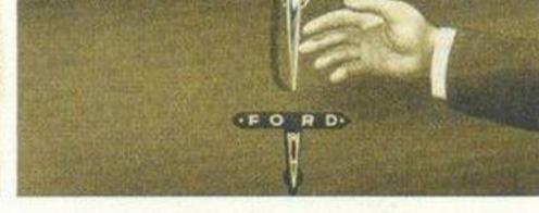
CENTRAL TAILGATE HANDLE. Allows easy, single-handed operation. When lowered on the plastic covered chains, the gate forms a useful loading platform - flush with the load-space floor.
