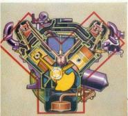
EVERY FEATURE MEANS MORE EFFICIENCY Overhead valves and double-deck intake manifold for more evenly distributed uel charges . . . Full turning intake and exhaust valves with integral guides for better performance and longer life . . . 3-ring super-fitted aluminiumalloy pistons step up power. . . . Highrigidity, Y-block design for smoother performance and longer engine life . . . Precision-cast crankshaft with five main bearings and eight integral counterweights for smoother operation.
