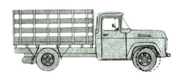
Big advantages in set-back front axle and wider track . . . The front axle is moved back providing a shorter wheelbase with greater manoeuvrability. Body load centre is moved forward and larger-capacity front axle supports a larger share of the load for better weight distribution. Wider track provides increased stability, and also provides the greater handling ease of Ford's turning angle of up to 39 degrees.
