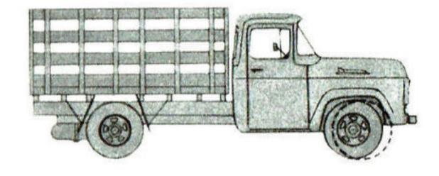
Big advantages in set-back front axle and wider track... The front axle is moved back providing a shorter wheelbase with greater manoeuvrability. Body load centre is moved forward and larger-capacity front axle supports a larger share of the load for better weight distribution. Wider track provides increased stability, and also provides the greater handling ease of Ford's turning angle of up to 39 degrees.
