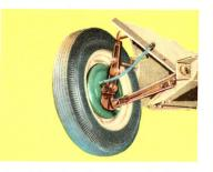
The independent front suspension is the well-proved torsion bar type, while the shock absorbers have been increased 5.6% in size to give a better ride and longer life. Two leading shoe front brakes ensure low pedal effort.
