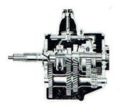
The 4-speed heavy-duty synchro-silent transmission is standard equipment on the  $3\frac{1}{2}$  ton Ford V8 F500. It provides more "pulling" ability plus more flexible and economical operation with heavy loads than 3-speed transmissions. It eliminates double-clutching and provides more safety in down shifting.
