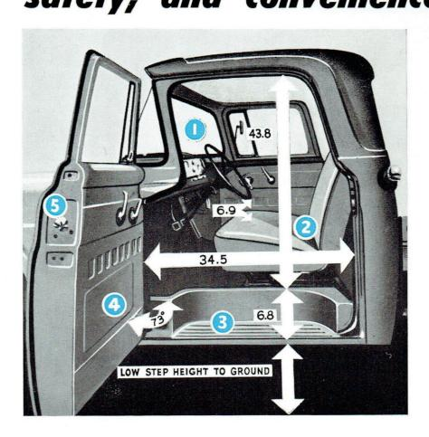
3. Inboard step. Ford has moved the cab step up inside the door making it easier to climb
