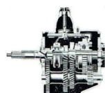
The 4-speed heavy-duty synchro-silent transmission is standard equipment on the  $3\frac{1}{2}$  ton Ford V8 F500. It provides more "pulling" ability plus more flexible and economical operation with heavy loads than 3-speed transmissions. It eliminates double-clutching and provides more safety in down shifting.
