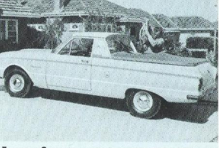
**Tonneau Cover** is completely water proof for full load protection. New design "tumble-action" hold-down clips are simplest to operate, **stay** closed under all conditions.
