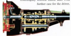
3-speed automatic drive. As an optional extra, fully automatic transmission is available. With fluid coupling on its three forward gear ranges, all changes are scarcely detectable.
