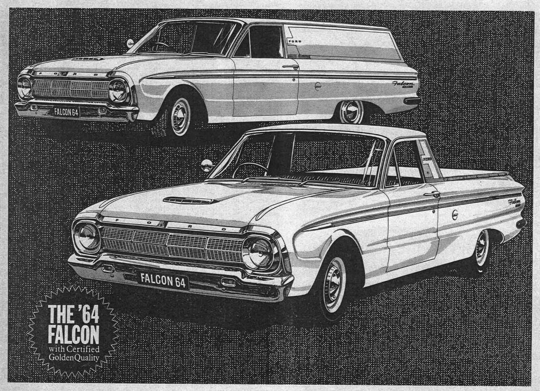
**NEW FALCON UTILITIES** — available in 2 models, standard and deluxe. With a capacity of 10½ cwt for payload and driver, they're the top load-carriers in their class. Features include double-steel wall construction around the load area, and two-stage rear suspension.
