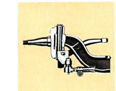
F 350's heat treated high carbon steel front axle has an increased 3,800 lbs. capacity. Its rigid I-Beam construction has increased strength at stress-point, and brenze kingpin bushings reduce friction and wear. There's extra strength in steering arms, knuckles and kingpins. Front axle shown viewed from the rear of the truck looking forward.
