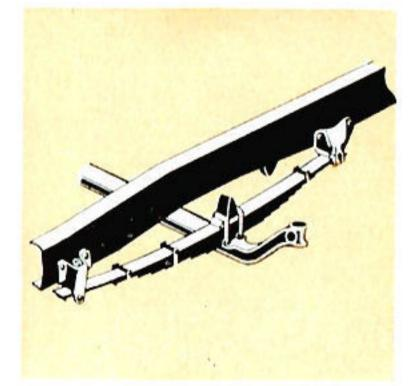
A better ride, empty or loaded, results from new front springs, which are stronger because at the front end the main leaf loop is supported by a half wrap of the second leaf. Double action shock absorbers are rubber insulated to deaden noise. Wide span, plus low deflection rate give most desirable riding qualities and stability.
