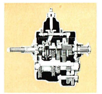
The "New Process 435" 4-speed synchrosilent transmission makes best use of F 350's power. New blocker-type synchronizers, integral with the mainshaft, give greater durability, and smooth, quiet gear engagement with little effort by the driver. provides more pulling ability and economical operation than 3-speed transmissions.
