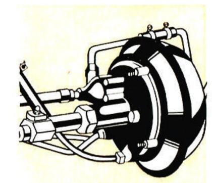
The heavy-duty hydraulic brakes, have had their total lining area increased to 238.04 inches. Internal shoe parking brake gives positive holding on steep inclines, supplements 4-wheel brakes in an emergency. You get the maximum stopping power on the move and the maximum security when standing stationary.
