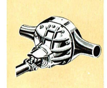
The rugged full-floating hypoid rear axle has a rated capacity of 7,400 lbs. Heathardened alloy steel construction prepares it to take shocks and strains, and more accurate ring gear alignment keeps it working for long periods without adjustment. All gears of alloy steel, heat treated for dependable strength and durability.
