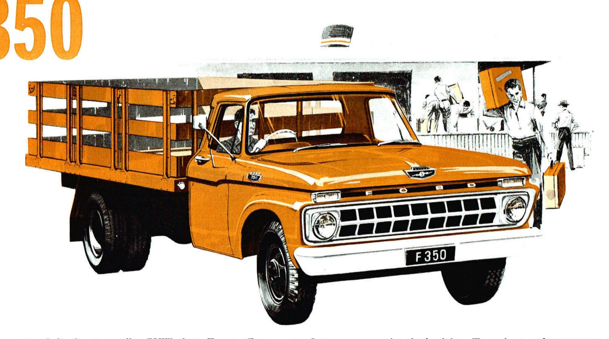
An entirely new truck in the 10,000 lbs GVW class, F 350 offers new performance and value. New performance comes from its entirely new 240 CID six cylinder engine and the all-new truck features detailed here. F 350's new value comes in offering all this
