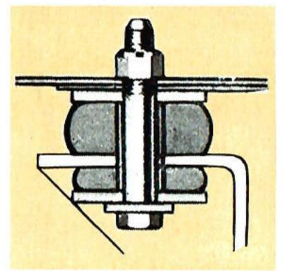
The system of rubber-cushioned 4-point cab mountings on Ford F-series trucks provide a better ride, and insulate the cab against frame stresses and vibration, reducing sheet-metal strains. The cab mountings accordingly improve the operator's comfort, increase cab life and maintain rigidity. They further add to F350's value for money.
