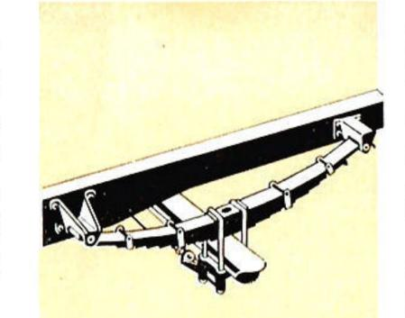
F 350 new variable rate rear springs are long and wide, with the correct resilience to handle the maximum load capacity under the most severe operating conditions. They give a smooth ride, loaded or unloaded. Their low deflection rate also adds to these desirable riding qualities, which greatly relieves operating fatigue.
