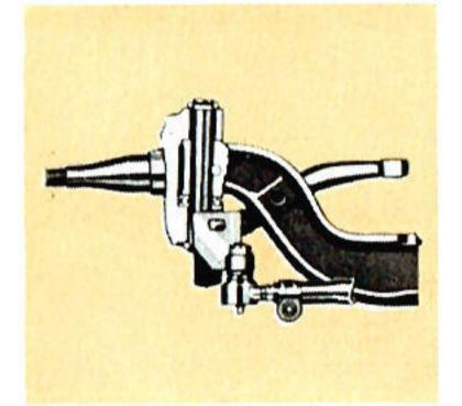
F 350's heat treated high carbon steel front axle has an increased 3,800 lbs. capacity. Its rigid I-Beam construction has increased strength at stress-point, and brenze kingpin bushings reduce friction and wear. There's extra strength in steering arms, knuckles and kingpins. Front axle shown viewed from the rear of the truck looking forward.
