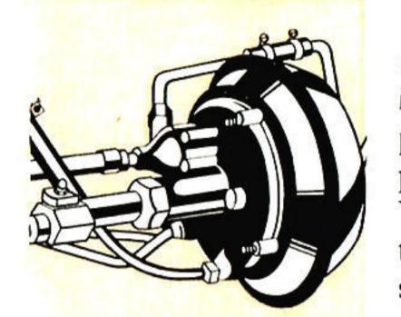
The heavy-duty hydraulic brakes, have had their total lining area increased to 238.04 inches. Internal shoe parking brake gives positive holding on steep inclines, supplements 4-wheel brakes in an emergency. You get the maximum stopping power on the move and the maximum security when standing stationary.
