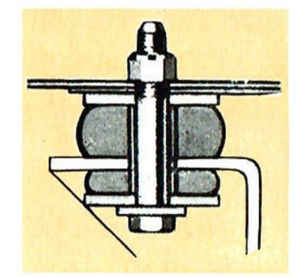
The system of rubber-cushioned 4-point cab mountings on Ford F-series trucks provide a better ride, and insulate the cab against frame stresses and vibration, reducing sheet-metal strains. The cab mountings accordingly improve the operator's comfort, increase cab life and maintain rigidity. They further add to F350's value for money.
