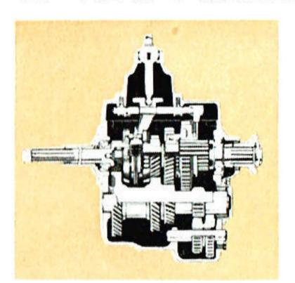
The "New Process 435" 4-speed synchrosilent transmission makes best use of F 350's power. New blocker-type synchronizers, integral with the mainshaft, give greater durability, and smooth, quiet gear engagement with little effort by the driver. It provides more pulling ability and economical operation than 3-speed transmissions.
