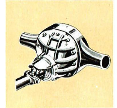
The rugged full-floating hypoid rear axle has a rated capacity of 7,400 lbs. Heat-hardened alloy steel construction prepares it to take shocks and strains, and more accurate ring gear alignment keeps it working for long periods without adjustment. All gears of alloy steel, heat treated for dependable strength and durability.
