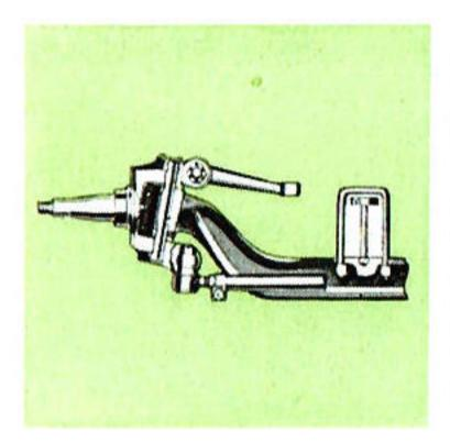
F 600's heat treated high carbon steel front axle has 6,000 lbs. capacity. Its rigid I-Beam construction has extra strength at stress-points, and delrin acetal resin kingpin bushings reduce friction and wear. There's big strength in steering arms, knuckles and kingpins. The front axle is illustrated from rear of truck, looking forward.
