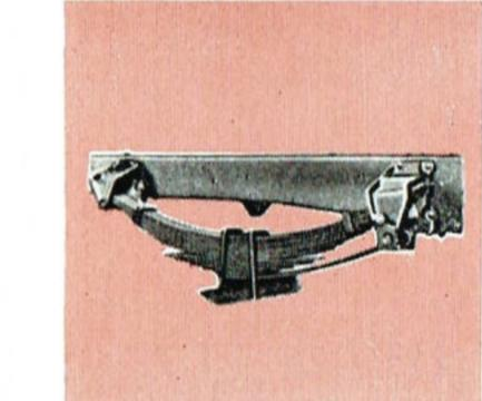
Front springs, of 2,700 lbs. capacity at pad are wide-span semi elliptics with low deflection rate. Rear semi-elliptic springs of 8,100 lbs. capacity use radius leaves to take driving thrust. This allows the main springs to perform their correct function, with desirable riding qualities and stability. They are built stronger, too.
