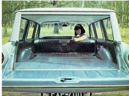
There are 77" of load length with the tailgate closed, 88" with it open.
