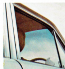
Laminated Windshield — with graduated tint for reduced daytime glare without reduced night vision.
