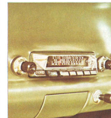
Push-button Radio — all-transistor, long range. Speaker mounted in top centre of instrument panel.
