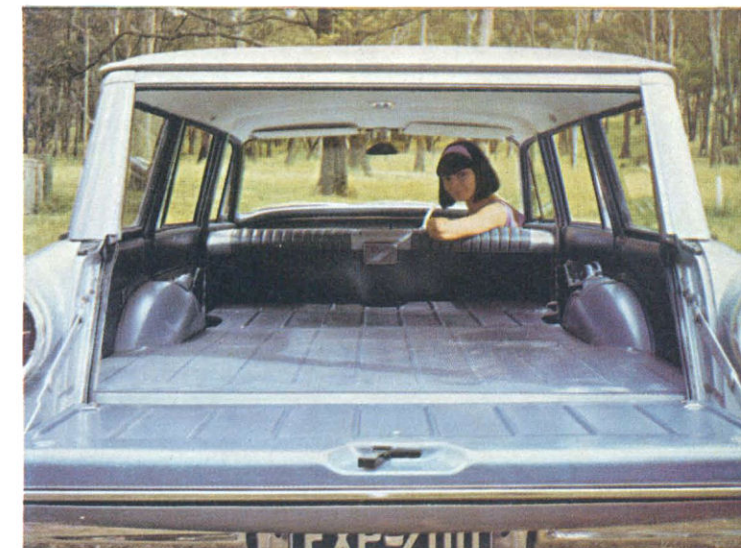
There are 77" of load length with the tailgate closed, 98" with it open.
