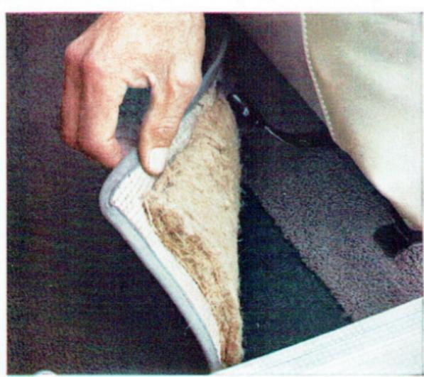
Insulating and sound-proofing materials completely surround the passenger compartment to absorb noise *before* it enters the interior. The engine hood, interior floor, and roof are lined. Undercoating, too, deadens road noise as well as protects Falcon's underbody against rust and corrosion.
