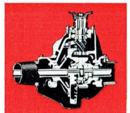
An extra-capacity 18,500 lbs Eaton spiral bevel full-floating 2-speed rear axle allows a combination of 10 forward and 2 reverse speeds, giving ideal ratios with desired flexibility for all road conditions and load variations. Ratio —7.17/9.77:1. This rear axle is matched to the tough work F800 has to do.
