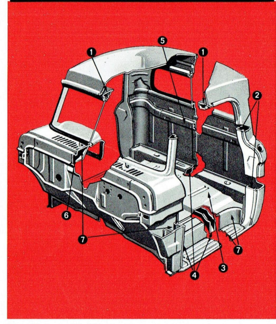
Long life is provided for Ford heavy-duty conventional cabs by allwelded construction and the following features:
