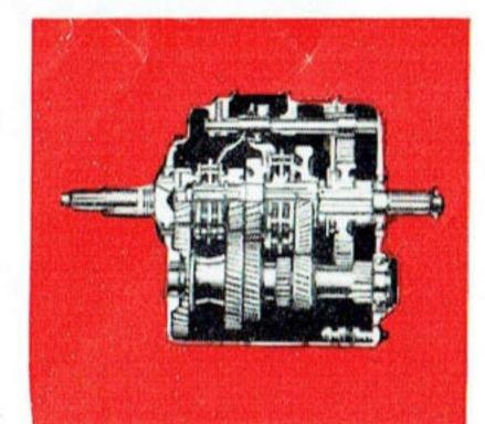
Ford F800's heavy-duty 5-speed Clark 2653-VI transmission is standard equipment. It has five forward and one reverse speed, with synchromesh on second, third, fourth and fifth. Constant mesh helical gears are fitted for the top four speeds. The transmission is one of the most proven in the business, with short gear travel in low and reverse.
