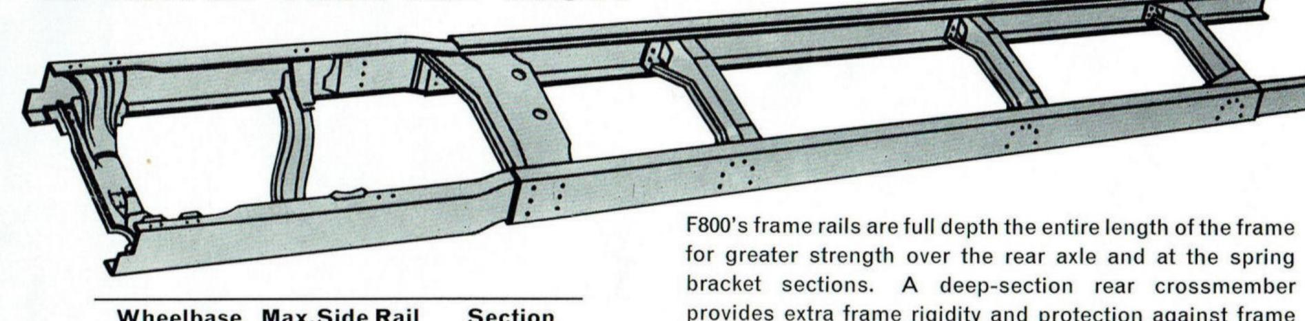
Wheelbase Max.Side Rail Section Modulus Section 9.56 x 3.06 x .28 158" 19.19 (Reinforcement 9.13 x 3.35 x .25 Inverted L)
