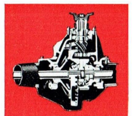
An extra-capacity 18,500 lbs Eaton spiral bevel full-floating 2-speed rear axle allows a combination of 10 forward and 2 reverse speeds, giving ideal ratios with desired flexibility for all road conditions and load variations. Ratio -7.17/9.77:1. This rear axle is matched to the tough work F800 has to do.
