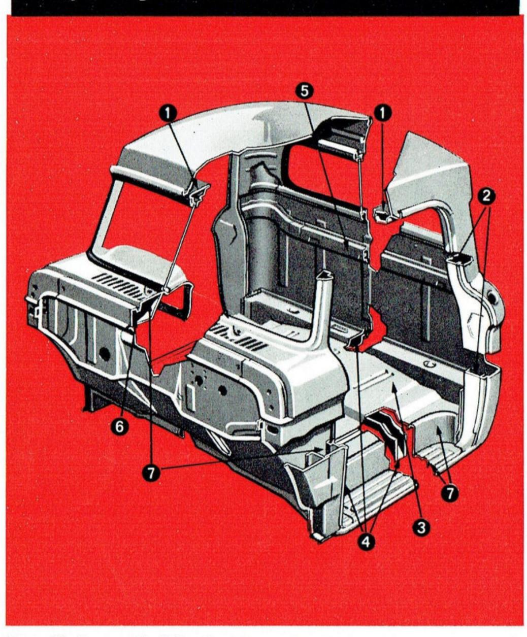
Long life is provided for Ford heavy-duty conventional cabs by allwelded construction and the following features:
