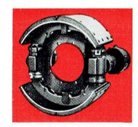
Powerful Heavy-duty hydraulic brakes have a total drum lining area of 641.9 sq. ins. with a big vacuum booster (including vacuum reservoir and warning light). Internal shoe parking brake gives additional security while stationary.
