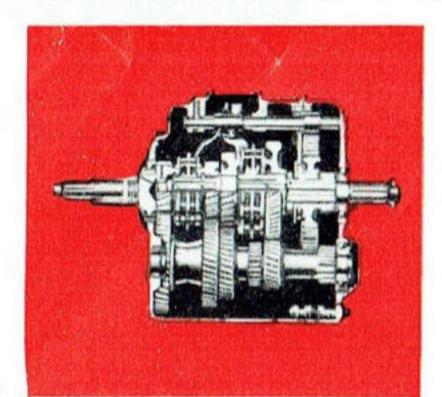
Ford F800's heavy-duty 5-speed Clark 2653-VI transmission is standard equipment. It has five forward and one reverse speed, with synchromesh on second, third, fourth and fifth. Constant mesh helical gears are fitted for the top four speeds. The transmission is one of the most proven in the business, with short gear travel in low and reverse.
