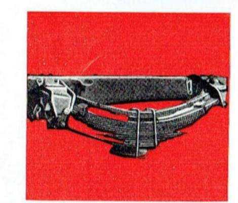
Front springs, of 4000 lbs capacity at pad, are wide-span semi-elliptics with low deflection rate. Rear main semi-elliptics have 9300 lbs capacity at pad, each using two radius leaves to take driving thrust. Fourleaf auxiliaries (also standard) have 2250 lbs capacity at pad.
