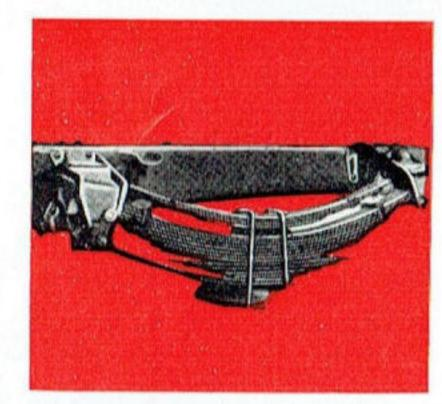
Front springs, of 4000 lbs capacity at pad, are wide-span semi-elliptics with low deflection rate. Rear main semielliptics have 9300 lbs capacity at pad, each using two radius leaves to take driving thrust. Fourleaf auxiliaries (also standard) have 2250 lbs capacity at pad.
