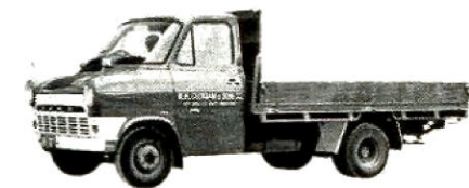
30 cwt. Cab Chassis with drop side body for general carrier utilization.
