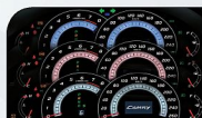
Optitron Combination Meter with Shift Position and MID (2.4 V & 3.5 Q Type) and Tri Color (3.5 Q Type)
