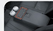
Rear Seat Controller for Audio, AC, Seat Reclining & Rear Sunshade (3.5 Q Type)
