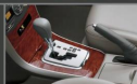
4 Speed Multi Mode Automatic Transmission, Gate Type with Sequential Shift (V & G Type)
