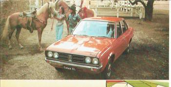
Galant XL. The Japanese favourite from Mitsubishi. A 1600 Saturn engine with a four speed box is backed up by disc brakes, plus MacPherson strut front suspension.
