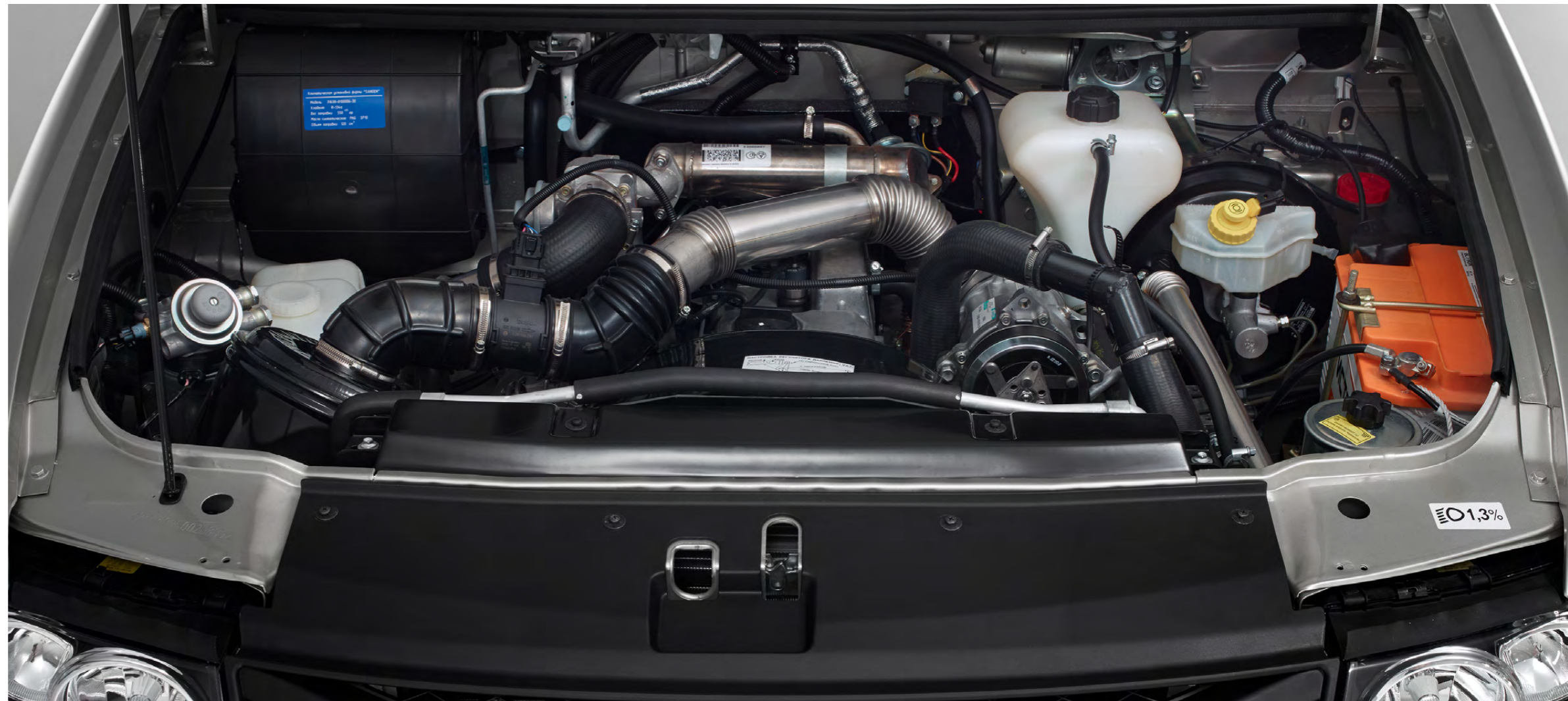
Diesel engine with 2.2 L displacement, 114 hp
