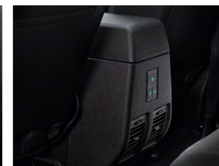
Control panel for additional heater and second-row seat heating
