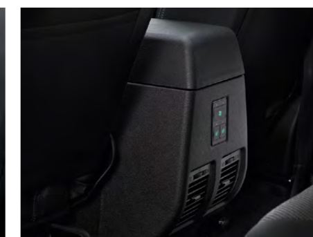
Control panel for air conditioning and heating
