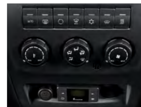
Control panel for air conditioning and heating
