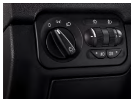
Light control panel
