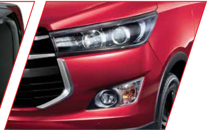
Automatic LED Projector Headlamps (with Follow Me Home Function), LED Daytime Running Lights (DRL) and Front LED Fog Lamps
