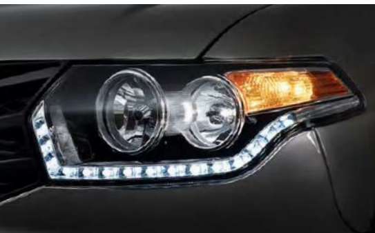
Headlamps with LED daytime running lights
