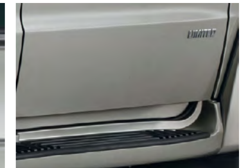
Body coloured integrated steps with nonslip cover
