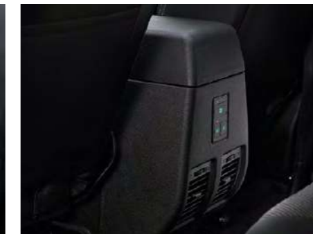
Control panel for air conditioning and heating
