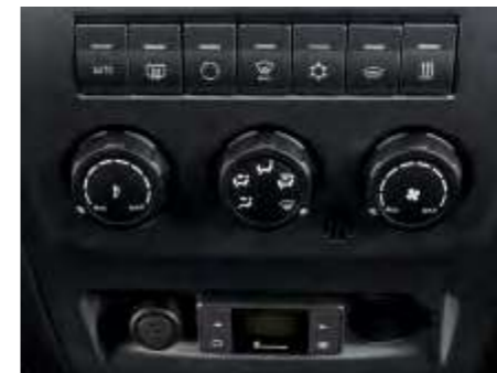
Control panel for air conditioning and heating
