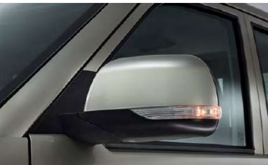
Large side mirrors with LED flashers
