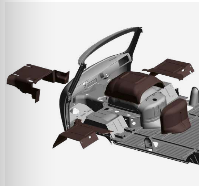
Improved vibration and acoustic comfort
