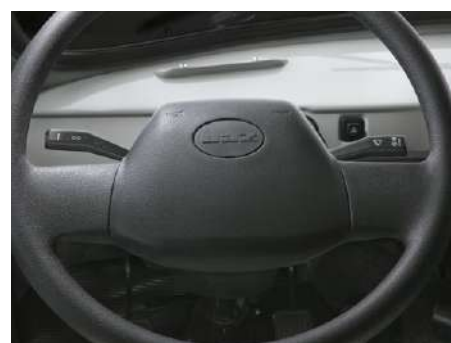
"Soft" steering wheel. Multifunctional Under-steering Switches
