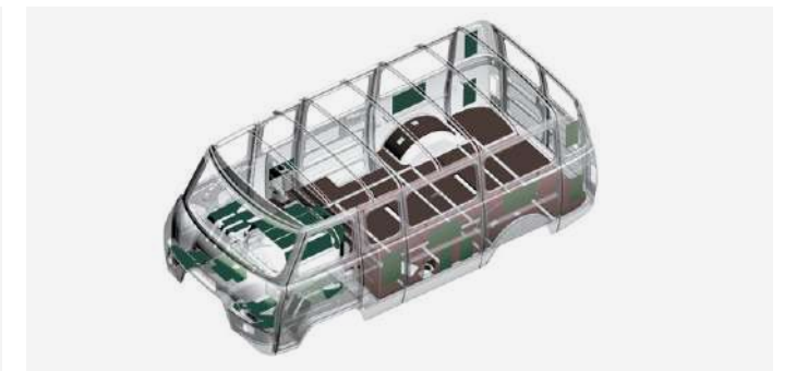
Improved vibration and noise insulation package all over the body, and special body-mounted pads
