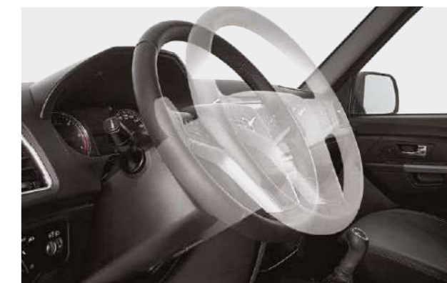
The new UAZ Patriot steering wheel can be adjusted both by tilt angle and height
