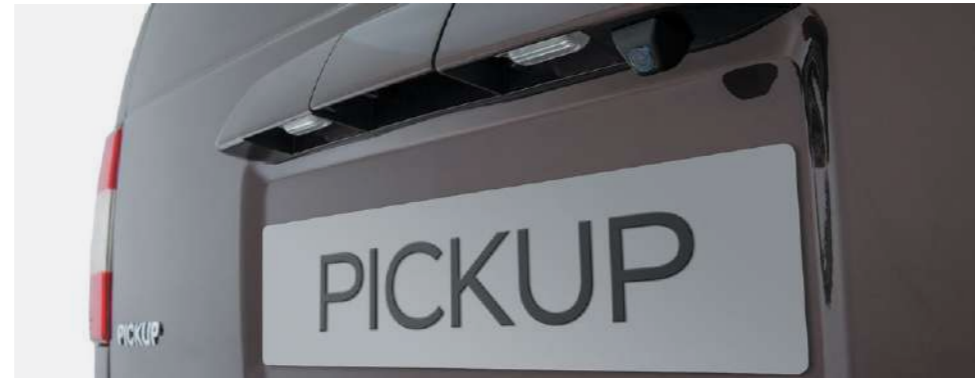
Rear view camera in the handle of the tailgate
