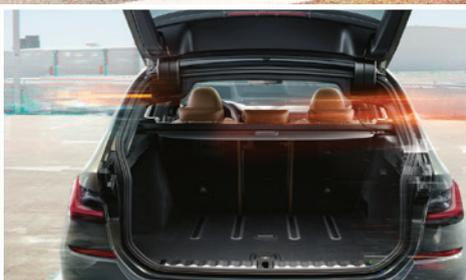
Clever luggage control. The standard Anti-slip rail system automatically creates friction with luggage, bags and suitcases, making them unlikely slide during driving or parking on slopes.
