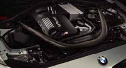
Expressive engine power. This champion 3.0-liter M TwinPower Turbo inline 6-cylinder delivers 411 horsepower, redlines at 7,600 rpms, and adds an extra punch of power with two turbochargers. The result is a screaming symphony of metal in motion that crescendos from 0-60 mph in only 4.2 seconds (M-DCT).
