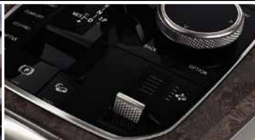
Adaptive 2-axle air suspension with automatic self-levelling suspension, selectable on five levels in total of 80mm adjustment travel
