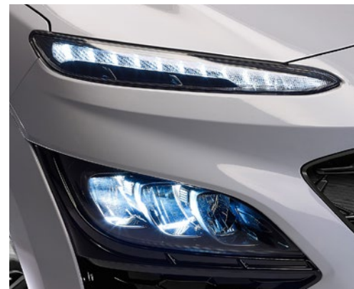
LED projection-type headlights (low and high)
