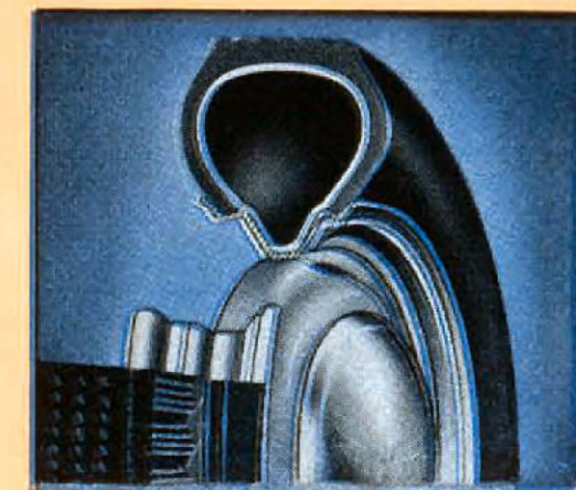
SAFETY-RIM WHEELS Help stop tyres from twisting off rims in case of blow-outs, allow safe, controlled stops.
