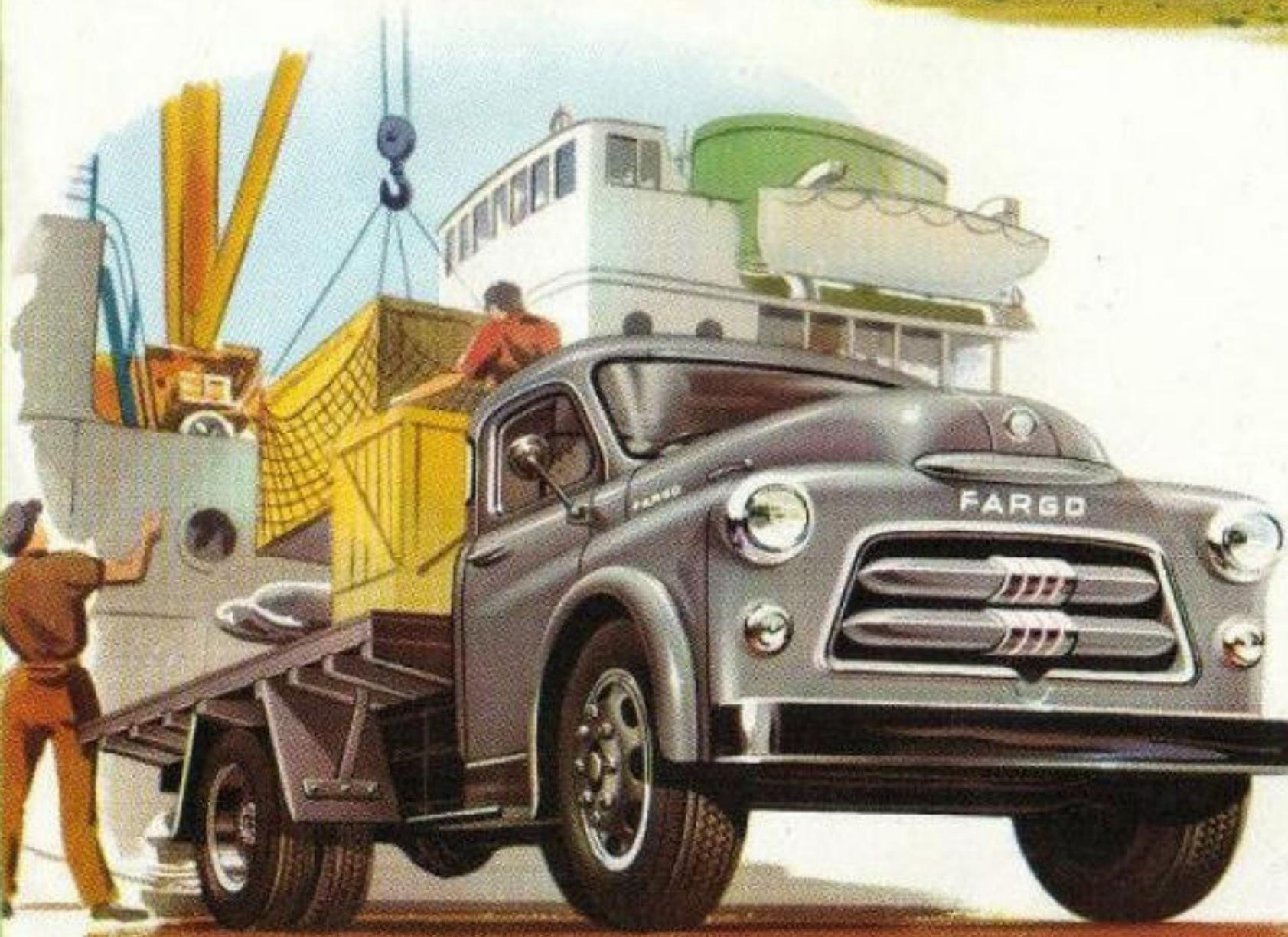
Here is the truck with every answer to every need in this payload range. The cab to axle dimension of 91" allows a big loading area without dangerous overhang of the body. The 250.6 cub. in. capacity engine with 5.85 to 1 ratio rear axle gives all the pulling power necessary for the load and with maximum economy. The powerful hydraulic braking system, incorporating two leading shoes on front wheels, adds to ease of handling — a particular benefit in city delivery work.
