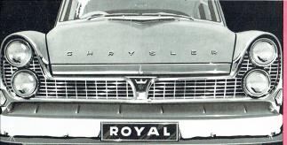
DUAL HEAD-LIGHTS: adding extra smartness to Chrysler Royal's front-end appearance, dual headlights provide added advantages for night driving. The two upper front headlights are double - filament sealed beam units, giving a low and high beam driving range. The lower headlights are single filament sealed beam units, used for high beam operation only.
