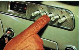
NEW TORQUEFLITE AUTOMATIC TRANSMISSION. This new, three-speed, push-button transmission is the last word in simplicity and safety. Push-button operation is provided for 1st, 2nd, Neutral, Drive and Reverse. Torqueflite is unusually smooth, extremely quiet, and gives amazing acceleration. As a safeguard against accidental selection, reverse gear cannot be engaged at speeds above 10 m.p.h.
