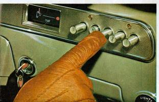
TORQUEFLITE AUTOMATIC TRANSMISSION. This three-speed, push-button transmission is the last word in simplicity and safety. Push-button operation is provided for 1st, 2nd, Neutral, Drive and Reverse. Torqueflite is unusually smooth, extremely quiet, and gives amazing acceleration. As a safeguard against accidental selection, reverse gear cannot be engaged at speeds above 10 m.p.h.
