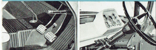
Above left: The easy-to-get-at clutch and brake pedals and "Orscheln" handbrake lever. Above right: Close-up of the safety-dished steering wheel and instrument cluster.
