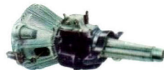
(17) All synchromesh 4-speed gear box. Toeboard mounted gearshift lever leaves the front floor unobstructed
