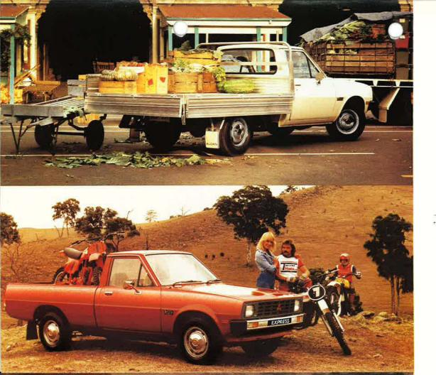
EXPRESS ONE TONNE CAB/CHASSIS. You won't find a 4-cylinder normal control cab/chassis as powerful as the Express. It has the 2.0 litre Astron engine and a 5-speed gearbox with gear ratios specially selected for performance and economy with or without a load. Build up this rugged hard worker any way you wish and you will haul loads up to 1000kg dependent on the body you choose.
