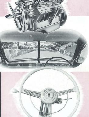
DIRECTIONAL SIGNAL AND SYNCHRO-AUTOMATIC GEAR SHIFT. The small lever at the right of the steering wheel signals a right or left turn by medium of the rear and parking lights. Turned upwards (i.e. in the leftwards direction of the wheel) it flashes the left-hand tail and parking lights. Turned downwards (i.e. in the right-hand tail and parking lights.—
