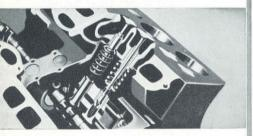
LA SALLE'S ANODIZED ALLOY PISTONS. The pistons are subjected to a special electrochemical both treatment which gives them a gem-like hardness despite their light weight. Advantages are: lighter weight, greater strength, and greatly minimized wear and scuffing, particularly when the engine is started from cold. — The T-slot type of piston will fit itself evenly and correctly within the cylinder bore throughout every change of operating temperature.
