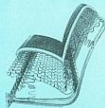
Holden's front and rear seating, with proven Z type, non-sag seat springs, gives a soft, comfortable ride. The front seat is designed to give excellent vision.
