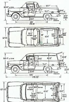
The new Holden Panel Van now has 77 cubic feet of space in its profit-making load area, which is now longer, wider and over four and a half inches higher for handling bulky goods.
