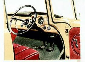
Inside the new Holden Panel Van you see the new instrument panel, new, dished steering wheel and hard-wearing, good-looking PVC upholstery and trim. Comfortable room for three is assured with "2" type springing and adjustable seat. The new windshield contains 1001.22 square inches of safety glass.
