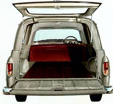
Increased load space means you can carry more goods more profitably than ever in the new Holden Panel Van. 77 cubic feet provide ample space for real payloads. There's good access for bulky loads through the new, wider and 71 inches deeper tailgate opening. Top and bottom tailgate hinging means easy load handling in the narrowest laneway.
