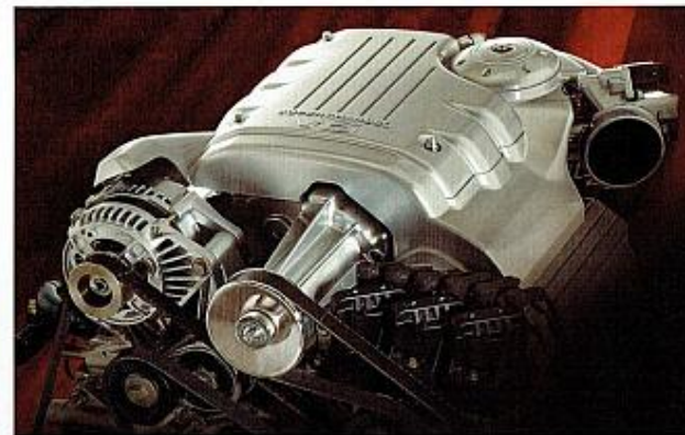
Supercharged V6 engine Both Commodore S and SS now offer the option of the powerful, yet efficient Supercharged V6 engine. This remarkable engine lets the Commodore S and SS driver enjoy the astounding performance gains of this elite technology, shared with Aston Martin, Jaguar and Mercedes-Benz. It now delivers 171kW of power and 375Nm of torque as the supercharger efficiently extracts peak power from premium unleaded petrol.
