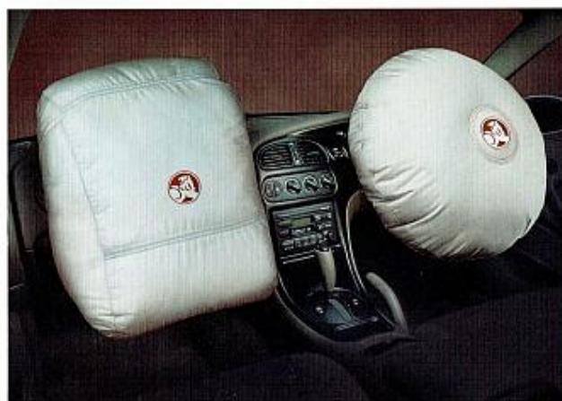
Driver and front passenger airbags The Commodore Acclaim features a driver and front passenger airbag system as standard equipment. These deploy simultaneously in milliseconds in conjunction with Commodore's front seat belt pre-tensioners. They also use 'tether' technology to prevent aggressive airbag injuries.
