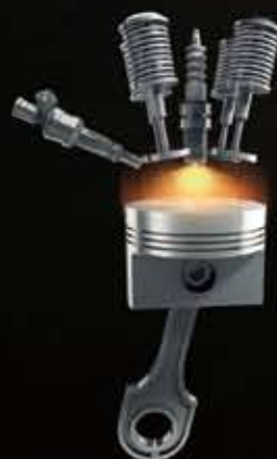
SIDI technology injects fuel directly into the cylinder, increasing power while saving fuel
