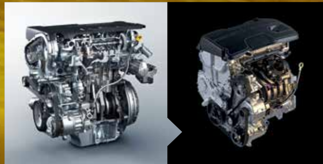
▲ 2.0L 4-cylinder common-rail turbo diesel engine ^
